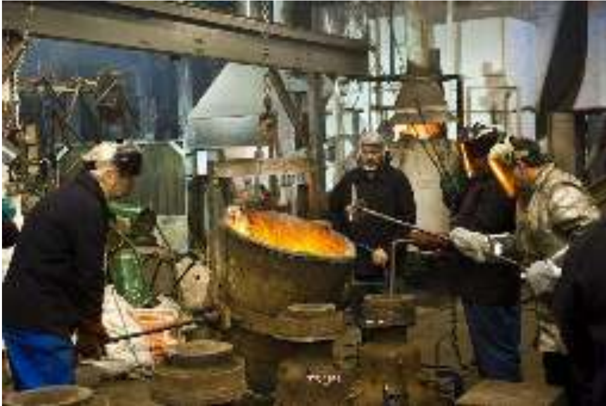
Whitechapel Bell Foundry, 32-34 Whitechapel Road, Tower Hamlets, London. Interior, casting room, filling the moulds.
