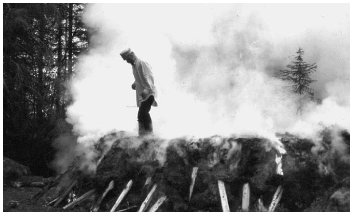
Fig. 8: Kiln for producing traditional wood tar. © NBA, Finland.
