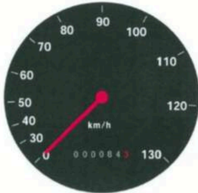
Figure 26 – an alternative design of a speedometer to capture change in the impact force Image Source: Rumar (1999)
